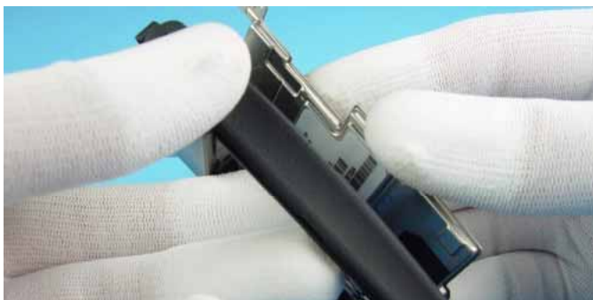
13) Remove the Shield from B-COVER.
