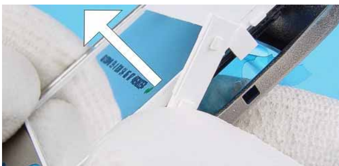
11) Press out the LCD MODULE while bending the C-COVER gently.
