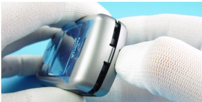
3) Press the A-COVER Lock before removing the B-Cover.
