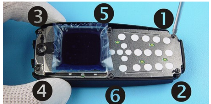
6) Remove SCREWS by using the shown order.
