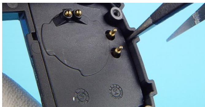
16) Unlock the plastic clips of the ANTENNA by use of tweezers.
