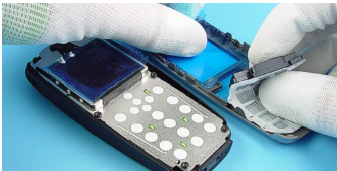
5) Remove KEYMAT, protect LCD and inner side window with a protective film.
