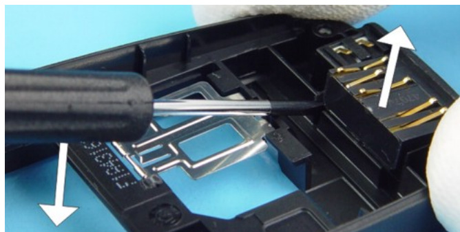
14) Use a slotted screwdriver as a lever to remove the SYSTEM CONNECTOR.
